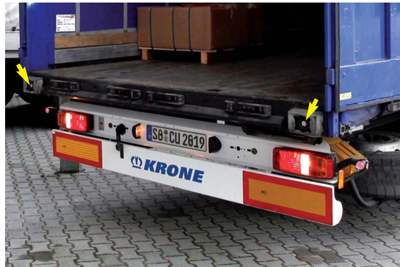
▶ TWO ULTRASOUND SENSORS DETECT THE CURRENT DISTANCE TO THE DOCK.
