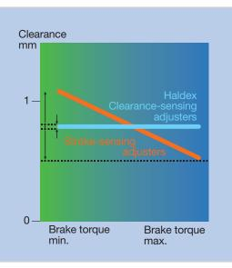
A Clear Winner: the Haldex S-ABA, a clearance-sensing brake adjuster provides a uniform constant distance between brake drum and lining, unlike the strokesensing brake adjuster – its clearance fluctuates with the application force of the brakes. drum. When the lining comes into contact with the brake drum, the adjusting mechanism disengages.
