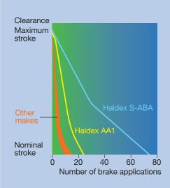
It also means that less clearance can be specified which results in a shorter piston stroke and in turn allows faster and safer brake application. A shorter stroke also enables the vehicle to use compressed air more efficiently.
