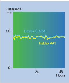
Clearance Comparison: The Haldex S-ABA and the earlier Haldex AA1 Brake Adjuster. The diagram (above) shows respective clearances between the drum brake and lining – the virtually identical graph lines show the high degree of clearance uniformity between the two brake adjusters.
