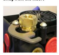
Once removed the o ring will be exposed. Replace with the new greased o ring
