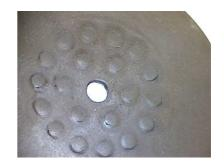
Examine the rubber diaphragm for any signs of damage or contamination and replace if required. Once diaphragm has been inspected / replaced then push in the park valve and check for leaks. If there is no leak, then re pipe chambers and check again.
