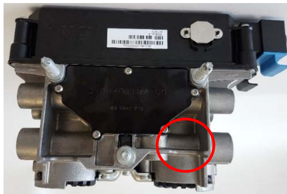
Picture 4 EB+ housing new modified without test port 21
