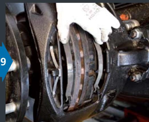
Use a file or wire brush to clean the shafts if necessary.
