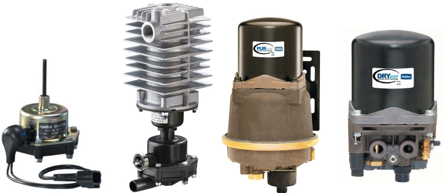
The Consep™ (Condenser/Separator) uses a simple, filterless design to separate and remove contaminants efficiently with minimal maintenance. The Automatic Drain Valve (ADV) automatically releases moisture from the tanks each time the brakes are applied as a first line of defense. The large volume desiccant cartridges of the DRYest™ and PURest™ simplify maintenance.
