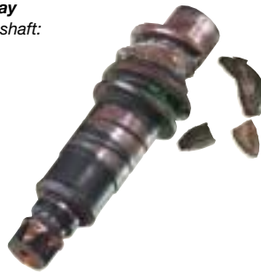
Three-way split This gearwheel copy broke before testing started.
