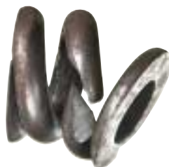
Worn out Deformed coil spring copy after 0.65 million applications.
