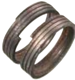
Non-starter Fragile clutch spring copy broke during installation.
