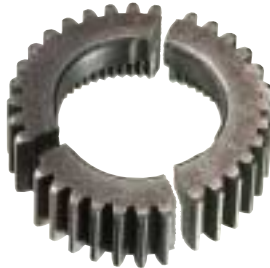
Three-way split This gearwheel copy broke before testing started.
