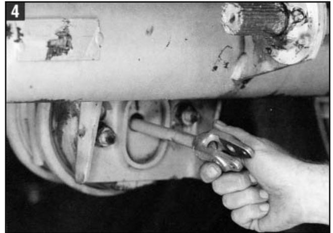
**4.** When installing a CSI Midland/Gunite automatic brake adjuster with a threaded clevis, install the new clevis on the push rod in the same locations as the clevis which was removed. Do not tighten the jam nut at this time.
