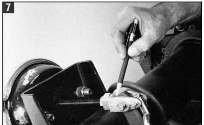
7. Before attaching the 1 1/4" collar nut to the clevis, check to make sure the threaded push rod is fully engaged in the 3/4" hex nut. If the push rod does not have full engagement, a new push rod must be installed and cut to length. Refer to the section on cutting a new push rod to length in this manual.
