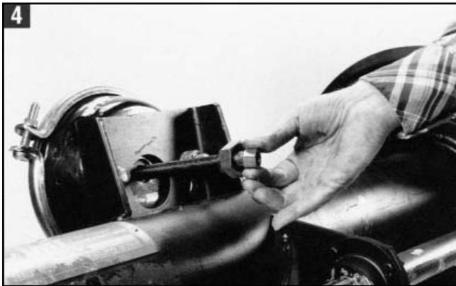
4. When installing a CSI Midland/Gunite automatic brake adjuster with a collar lock clevis, place the 1 1/4" collar nut on the push rod against the 15/16" jam nut. Next thread the 3/4" jam nut onto the push rod.
