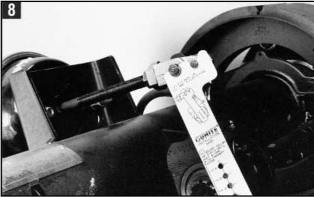
8. After threading the 1 1/4" collar nut onto the clevis housing, place the template over the large and small clevis pins as shown above.
