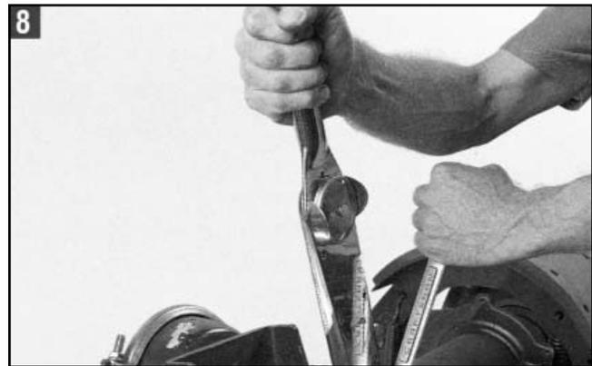
8. Tighten the jam nut against the clevis housing using 40 to 50 ft lbs of torque. If you do not tighten the jam nut now, it will allow the clevis to rotate freely and change the position of the clevis resulting in an improper installation.
