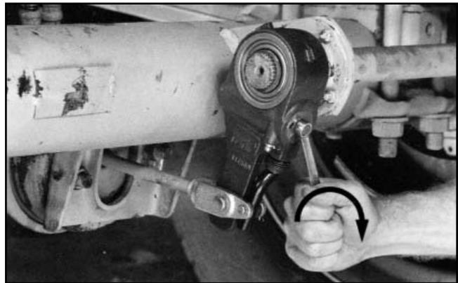
7. Once the linings have been replaced and the brake drum installed, rotate the adj hex clockwise until the brake linings contact the brake drum.
