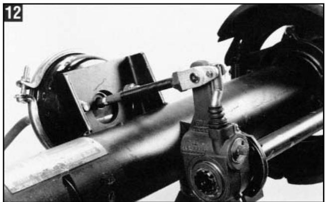
12. Fully apply the brakes and allow the chamber push rod to travel its maximum stroke. Clearance must exist between the brake adjuster and all adjacent chassis components. Release the brakes.
