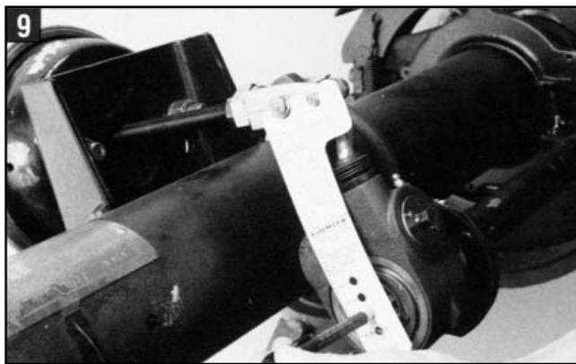
9. Align the brake adjuster by adjusting the 3/4" hex nut on the push rod until the appropriate centering hole on the template aligns with the center hole on the camshaft. The template is provided with centering holes for 5, 5.5, 6 and 6.5 inch brake adjusters.
