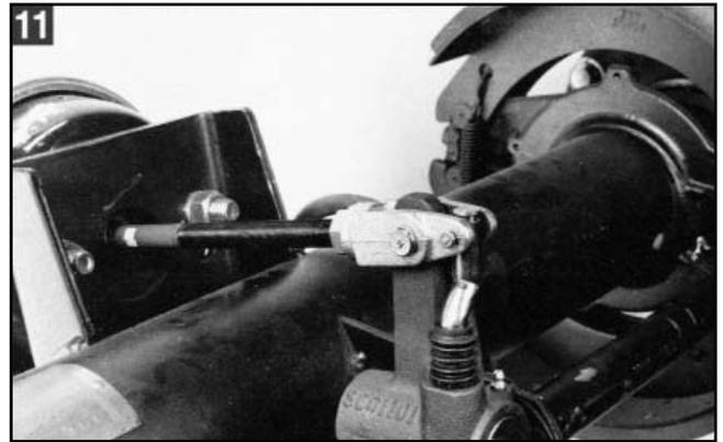
11. Fully apply the brakes and allow the chamber push rod to travel its maximum stroke. Clearance must exist between the brake adjuster and all adjacent chassis components. Release the brakes.
