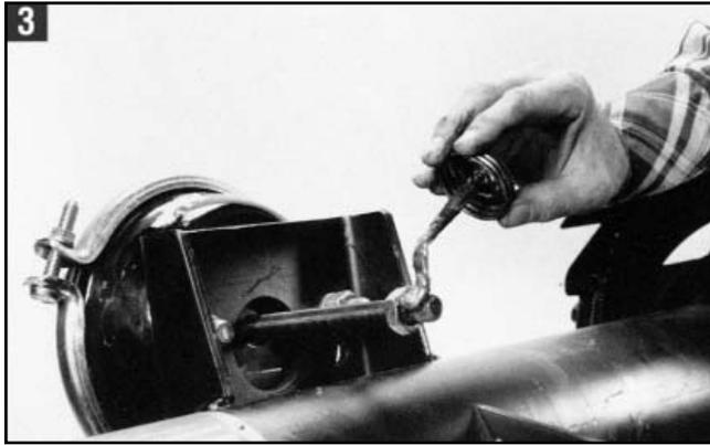
3. Apply anti-seize to the chamber push rod threads before installing the new clevis. Also apply anti-seize to the camshaft splines at this time.
