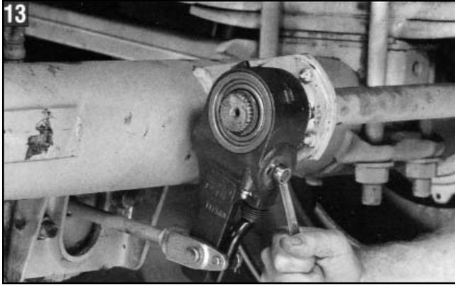
**13.** Pre-adjust the brakes by rotating the adjust hex clockwise until the brake lining contacts the brake drum. Back the brake adjuster off by rotating the hex counterclockwise 1/2 turn. Backing off a new brake adjuster may require up to 50 ft lbs of torque. A ratcheting sound will be heard when backing the brake adjuster off.
