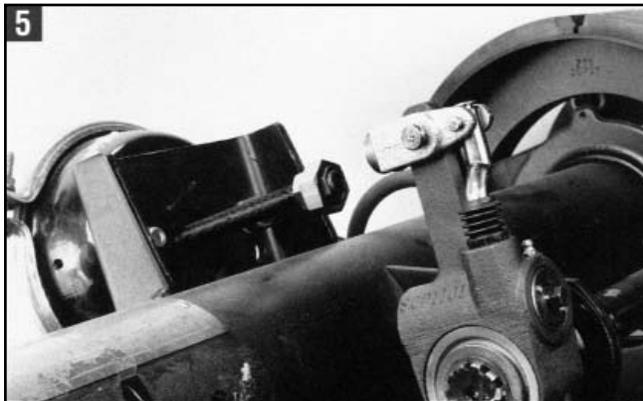
5. Install the brake adjuster onto the camshaft with the adjusting hex pointing away from the brake chamber. Secure the brake adjuster on the camshaft. Use at least one inner washer and enough outer washers to allow no more than .060 movement of adjuster on camshaft. (Per TMC recommended practice RP609-A). **NOTE: Do NOT pull push rod out to meet the brake adjuster.** Rotate the 7/16" adjusting hex nut CLOCKWISE.
