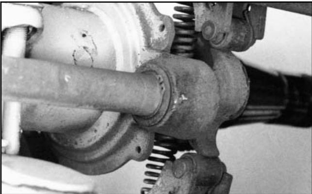
5. After the brake drum has been removed; rotate the adj hex clockwise until the cam turns over. This will allow the brake rollers to be in the release position.
