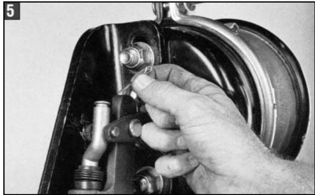
5. Insert the cotter pins into the large and small holes and secure the cotter pins.
