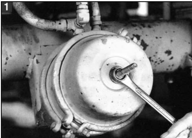
1. If the axle is equipped with spring brake chambers, manually cage the spring brakes following the manufacturer's recommended procedures. Note: When caging the spring brakes, always be sure to block the vehicle wheels to prevent unwanted movement.
