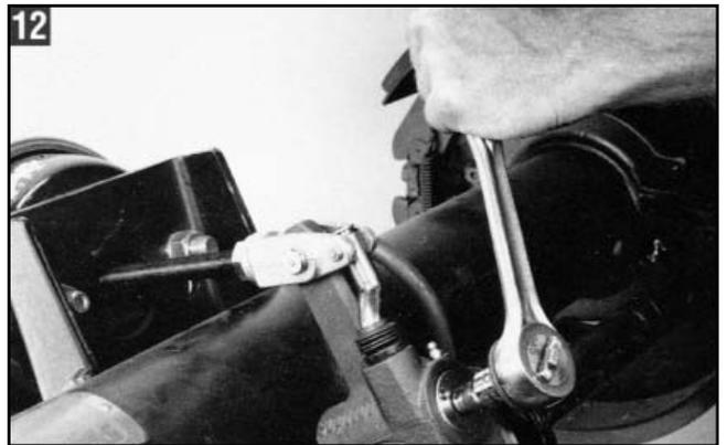
12. Pre-adjust the brakes by rotating the adjust hex clockwise until the brake lining contacts the brake drum. Back the brake adjuster off by rotating the hex counterclockwise 1/2 turn. Backing off a new brake adjuster may require up to 50 ft lbs of torque. A ratcheting sound will be heard when backing the brake adjuster off.
