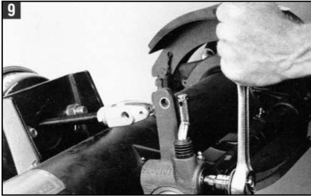
9. Apply anti-seize compound to the camshaft and clevis pins. Install the brake adjuster onto the camshaft with the adjusting hex pointing away from the brake chamber. Secure the brake adjuster on the camshaft. Use at least one inner washer and enough outer washers to allow no more than .060 movement of adjuster on camshaft. (Per TMC recommended practice RP609-A). **NOTE: Do NOT pull push rod out to meet the brake adjuster.** Rotate the 7/16" adjusting hex nut **CLOCKWISE**.
