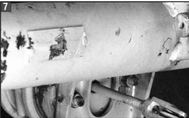
7. Inspect the clevis installation to make sure the threaded push rod extends no more than 1/16" past the end of the opening of the clevis in the clevis housing. If the push rod extends more than 1/16" past the clevis opening, mark the push rod and remove the clevis to allow the push rod to be cut to the proper length.
