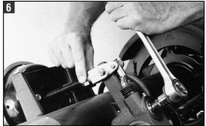
6. Using the hex extension and a wrench, adjust the brake adjuster so that the collar nut aligns with the threaded area of the clevis.
