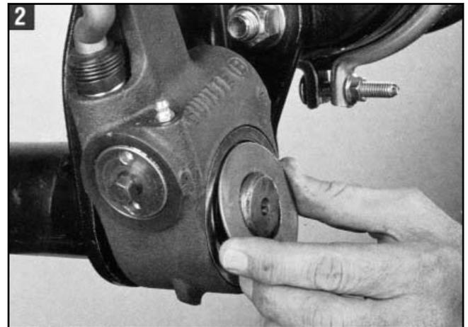
2. Apply anti-seize compound to the camshaft splines. Install the brake adjuster onto the camshaft with the adjusting hex pointing away from the brake chamber. Secure the brake adjuster on the camshaft. Use at least one inner washer and enough outer washers to allow no more than .060 movement of adjuster on camshaft. (Per TMC recommended practice RP609-A). **NOTE: Do NOT pull push rod out to meet the brake adjuster.**
