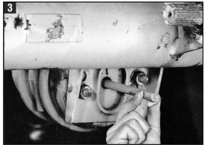
**3.** Apply anti-seize to the chamber push rod threads before installing the new clevis.
