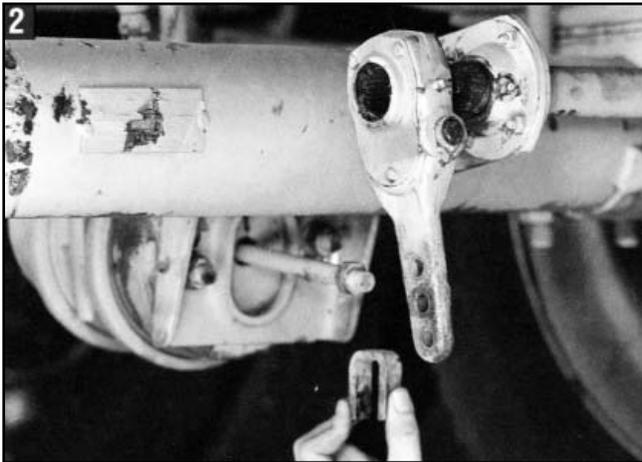
**2.** Remove the existing clevis and brake adjuster. Keep the existing mounting hardware. Do not remove the clevis jam nut.
