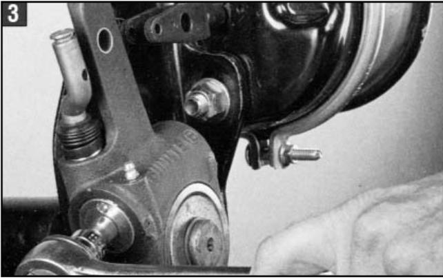
3. Using a 7/16" wrench or a socket, rotate the adj hex clockwise until the holes in the brake adjuster are properly aligned with the corresponding holes in the welded clevis.
