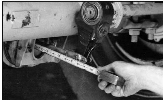
9. Using a ruler, measure the distance from the face of the air chamber to the center of the large pin in the clevis (A). (See Figure 15.)
