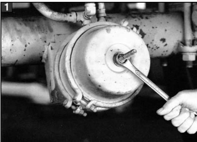
1. Block the vehicle's wheels. If the axle is equipped with spring brakes, manually cage the brakes following the manufacturer's recommended procedures.
