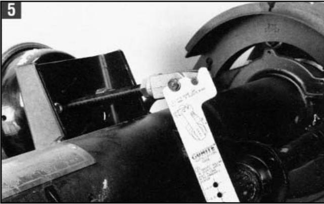
5. Once the clevis has been installed on the threaded push rod, install both the large and small clevis pins. Now position the installation template over both the large and small clevis pins.
