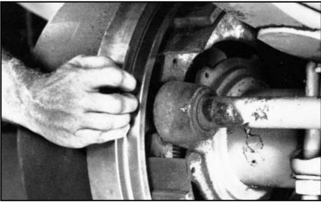
4. Only back off the adjusting hex enough to allow the drum to clear the lining. Remove the brake drum.
