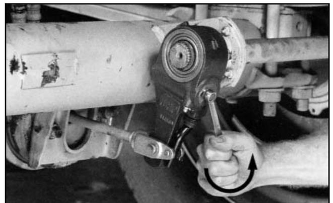
3. Using a 7/16" wrench or socket, rotate the adj hex counterclockwise. You should have at least 15 ft. lbs. resistance and a ratcheting sound will be heard as the adj hex is rotated.
