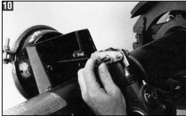
10. Once the clevis is properly aligned with the brake adjuster, insert both the large and small clevis pins and secure with the cotter pins supplied.
