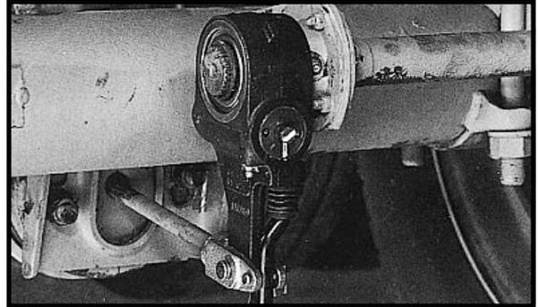
Figure 9 - Brake Adjuster Function
