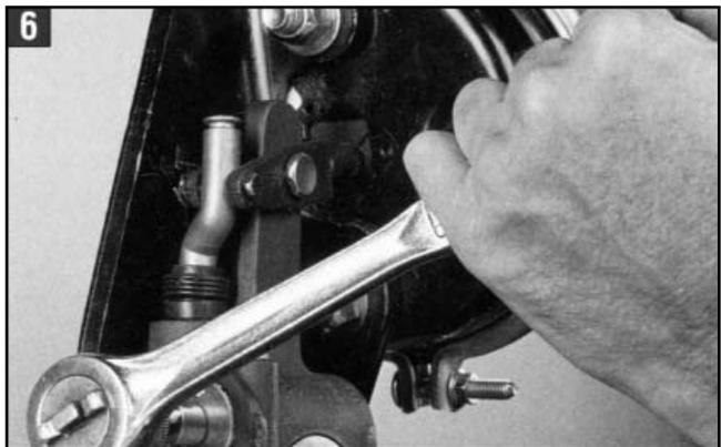
6. Pre-adjust the brakes by rotating the adjust hex clockwise until the brake lining contacts the brake drum. Back the brake adjuster off by rotating the hex counter-clockwise 1/2 turn. Backing off a new brake adjuster may require up to 50 ft lbs of torque. A ratcheting sound will be heard when backing the brake adjuster off.
