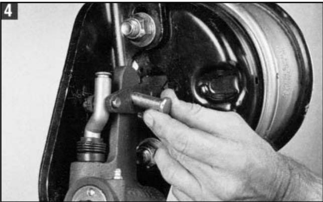
4. Apply anti-seize compound and insert the large and small pins in the proper holes.
