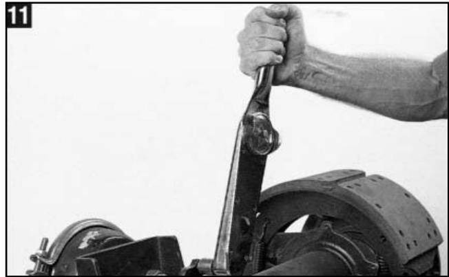
11. Once the 1 1/4" collar nut has been properly tightened to the clevis, tighten the 15/16" jam nut against the collar lock nut using 40 to 50 ft lbs of torque.
