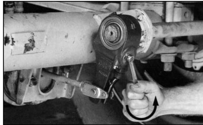
8. Back-off the brake adjuster by rotating the adj hex 1/2 turn counterclockwise. A ratcheting sound will be heard. This will provide running clearance between the lining and the drum's braking surface.
