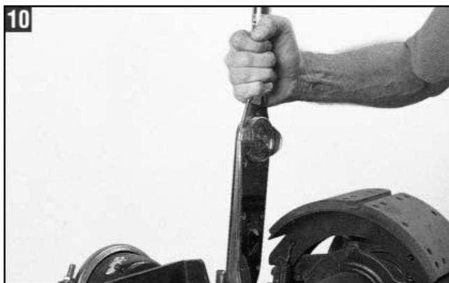
10. Using a torque wrench, tighten the 1 1/4" collar nut to the clevis using 40 to 50 ft lbs of torque.
