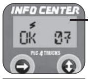
From the active fault screen, CODE 07, vehicle is stationary ABS is fully operational.
