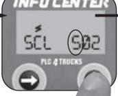
Hold the right button for two seconds. The first digit will begin flashing.
