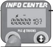
Press the left button to display the odometer. Example: 18.7 miles
