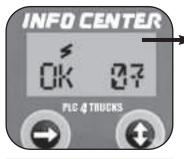
From the active fault screen, CODE 07, vehicle is stationary; ABS is fully operational.
