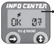
From the active fault screen, CODE 07, vehicle is stationary; ABS is fully operational.
