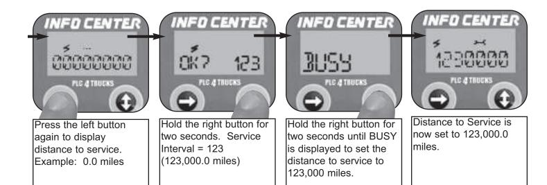
The Distance to Service is the Service Interval Counting Down. Once it reaches zero, service is required. The Trailer ABS Warning Lamp will flash three times on power up until distance to service is set again or until a new service interval is set.
