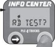
Hold the right button for two seconds. Request to test the red valve channel. (Red if 2S/1M)
