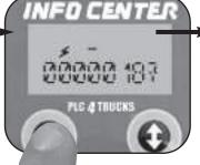
Press the left button to display the odometer. Example: 18.7 miles
