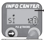
After setting all three digits, hold the right button for two seconds until BUSY is displayed. Service Interval is set to 123 = 123,000.0 miles.
