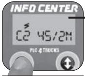
Press the left button again to view Sensor/ Valve ABS configuration. Example: C2 = 4S/2M (4 Sensors/2 Modulator Valves)
