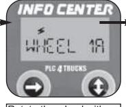
Rotate the wheel with sensor 1A (1 Rev/2 Sec) four seconds minimum.
