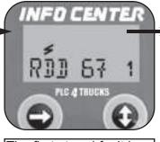
The first stored fault is displayed. Example: 67 fault, occurred 1 time. If OK 00 is displayed, no stored faults are present.
