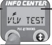
Press the left button to display VLV TEST.
