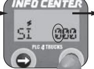
Hold the right button for two seconds. The first digit will begin flashing.
