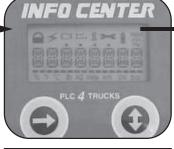
Next screen displays an all Segment Display Test.
