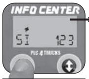
Press the left button again to display the service interval. Example: SI 123 SI is 123,000 miles
