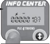
Press the left button again to return to the odometer.
