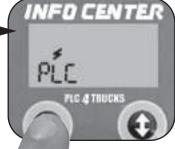
Press the left button to view ABS Type "PLC", "PLC SLCT" or "PLC PLUS".
