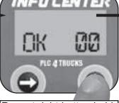
Repeat right button hold to clear stored fault codes. Otherwise wait to return to the active fault screen.
