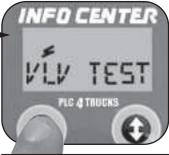
Press the left button to display VLV TEST.
