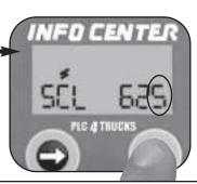
After setting all three digits and the mile or km icon. hold the right button for two seconds until BUSY is displayed. The Tire Scale Factor is now set. Example: 625 rev/mile.
