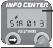
The next stored fault is displayed. Example: 01 fault, occurred 3 times. Repeat right button hold for two seconds until BUSY is displayed.
