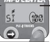
Press the right button to set the first digit (0 - 9). Service Interval is in 1,000 mile increments. Example:100 =100,000 miles
