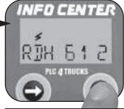
Repeat right button hold for next stored fault. Example: 61 fault, occurred 2 times. Repeat right button hold for two seconds until BUSY is displayed.
