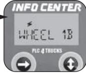
Rotate the wheel with sensor 1B (1 Rev/2 Sec) four seconds minimum.
