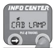
The display returns to CAB LAMP. Press the right button to repeat the in-cab lamp test. Press the left button to return to display WHEEL.
