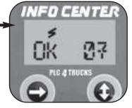
After clearing stored faults, the display returns to the active fault screen.
