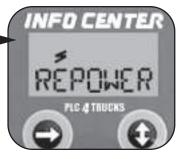
After the valve is tested, the ABS will not be functional. Re-power the ABS System.
