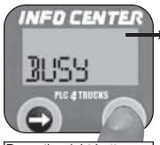
Press the right button until BUSY is displayed. The red channel valve is energized. The ABS Warning Lamp will begin to flash.
