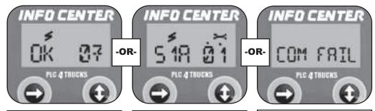
If powers up to an 07 code, vehicle is stationary. ABS is fully operational. If trailer ABS lamp is still ON, check stored faults. (See Pages 1-5 for complete fault code list.)
