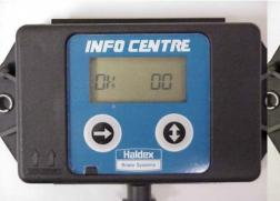
Repeat Right Button Hold to Clear Stored fault Codes. otherwise wait to return to the Active Fault Screen.
