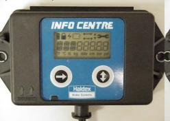
Press the Left Button Again To View Segment Display Test
