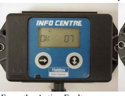
From the Active Fault screen, Code 07, Vehicle is Stationary ABS Fully Operational
