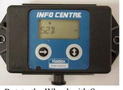
Rotate the Wheel with Sensor 2B (1 rev/ 2 sec) 4 sec min. 2B will remain Displayed
