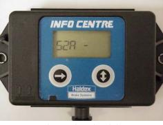
Rotate the Wheel with Sensor 2A (1 rev/ 2 sec) 4 sec min. S2A will remain Displayed
