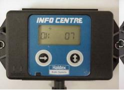
From the Active Fault screen. "OK 07", Vehicle is Stationary ABS is Fully Operational
