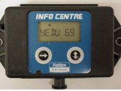
The First Stored Fault is Displayed. Example: "Yedu 69" Fault
