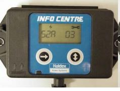
Repeat Right Button Hold for Repeat Right Button Hold until next Stored Fault. Example: "S2A 03" Fault
