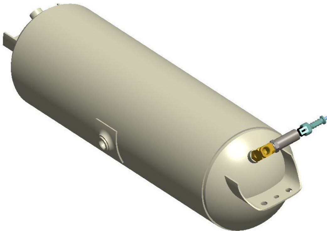
Figure 2: External Pressure Sensor Transducer plumbed into the air reservoir.
