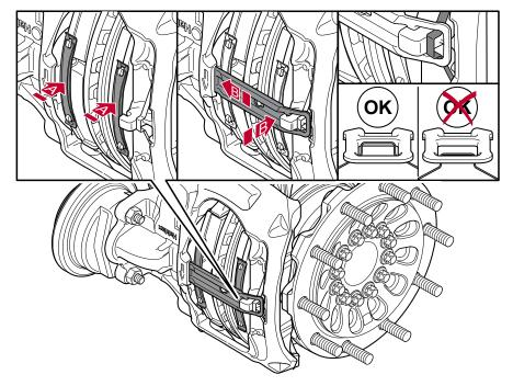
Install new pad springs and pad retainer
