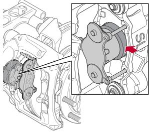
Inspect the thrust plate bellows.
