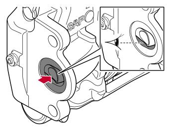
Inspect ball cup and seal of brake chamber lever.
