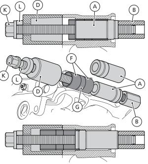
Remove the leading slide bearing.
