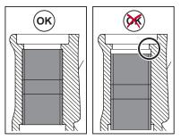
Leading slide bearings installed.
