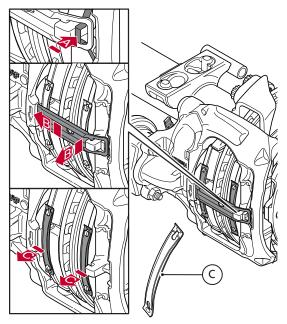
Remove pad retainer and pad springs.
