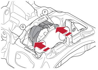
Press in the thrust plate bellows.
