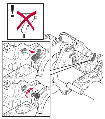
De-adjustment of the reset shaft.
