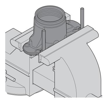
Clamping arrangement for thrust plate.
