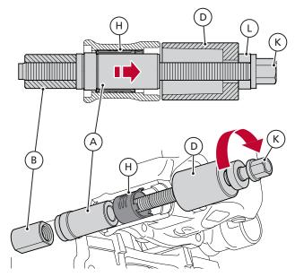
Remove the trailing side composite bearing.
