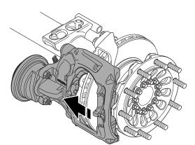
Push brake caliper to inner position.
