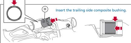
If the bushing is not indexed correctly, the slide pin and protective cup may not fit.
