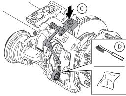
Place dial indicator on carrier. Clean the measuring point.
