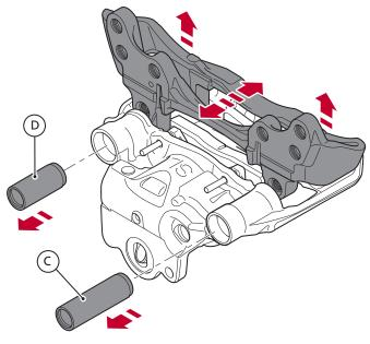
Remove the carrier and slide pins.
