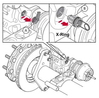
Remove the reset shaft.
