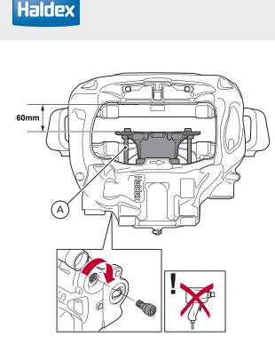
Extend thrust plate for bellows inspection.
