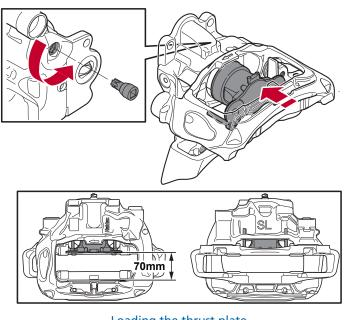
Loading the thrust plate.
