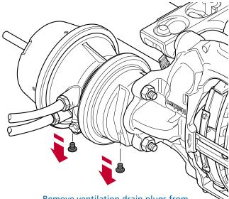
Remove ventilation drain plugs from bottom side of spring brake chamber.
