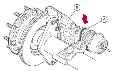
Clean mating surfaces of brake and chamber.
