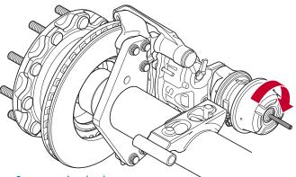
Secure spring brake in the active position.
