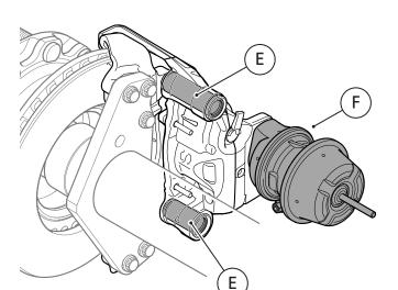
Slide pins and spring brake chamber.
