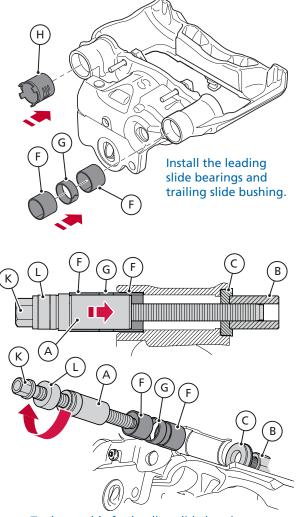
Tool assembly for leading slide bearings.
