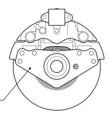
The ModulT Gen II is a directional caliper. It is important that the correct caliper is installed in relation to the normal wheel / rotor rotation. Each caliper has a rotation arrow cast on the surface of the caliper where the pad retainer seats on the inboard side. Illustration provides a general overview with the rotation shown with a red arrow and the leading slide pin (AL) and the trailing slide pin (AT).
