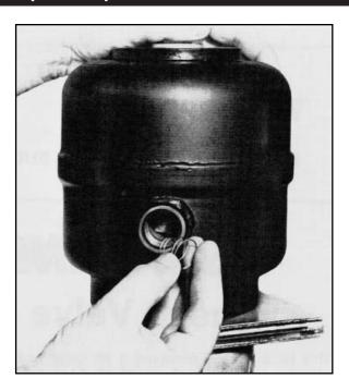
**Step 4:** Place the new spring in back of the poppet (with small end of spring facing poppet).
