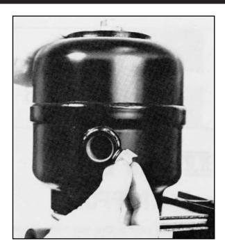
**Step 3:** Place the O-Ring/poppet assembly into the check valve body, O-Ring end first, as shown. Needle nose pliers may be used to guide the poppet into place.
