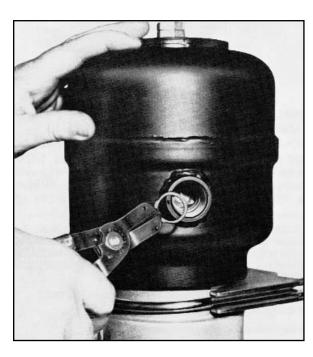
**Step 1:** Loosen the connections at the inlet and outlet of the air dryer and bleed the system. After relieving the air system pressure, remove the hose line and/or adapter from the 3/4" female NPTF outlet port. Remove the retaining ring (item 4) with snap ring pliers. Remove the spring (item 3) and poppet O-Ring assembly (item 2 and 1).
