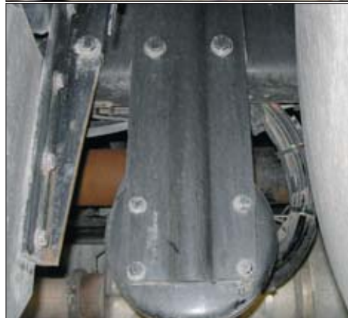
Inside of Frame Rail Installation. Uses Air Dryer Mounting Bracket (Item 1) and Tank Mounting Bracket (Item 19) which orients the Air Reservoir/Purge Tank (Item 12) vertically.
