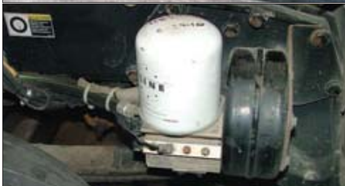
Photo showing the Bendix® AD-IS mounted on the vehicle. The dryer is located in front of the steer axle on the passenger's side.
