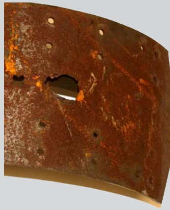
Rusted Holes in Shoe Table
