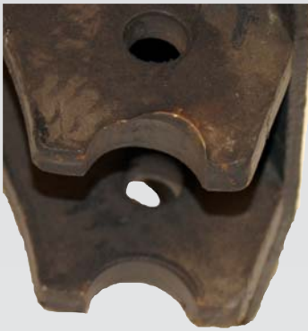
Flared and Damaged Cam Ends
