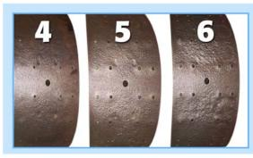
Cores with quality grades of 4, 5 or 6 are automatically culled from the production process and scrapped. These cores exhibit characteristics that will shorten the life cycle of the shoe and have a high potential to prematurely corrode. Rivet holes are often out of spec.
