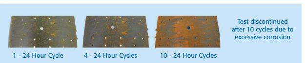
Summary Analysis: Corrosion present after just one cycle of testing. This indicates that the cure process is substandard. Corrosion remains consistent between cycles 1 and 4. This indicates the paint is somewhat stable at these early stages. Corrosion explodes between cycles 4 and 10. This indicates that the paint destabilized pervasively during this period.
