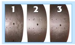
Cores with quality grades of 1, 2 or 3 are initially deemed acceptable to continue through the remanufacturing process. These cores will exhibit tables that are in excellent condition. They would not have been exposed to excessive corrosion or other damage. Rivet holes are symmetrical.
