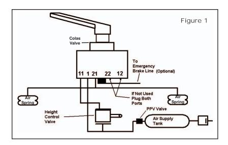
**Note:** There are two sets of supply and delivery ports on the Colas Valve. Both may be used at the same time, but if only one set is used the other must be plugged or the valve will not operate properly. Port 11 (from HCV) corresponds with delivery port 21 and Supply port 12 (from HCV) corresponds with delivery port 22 on the Colas Valve.
